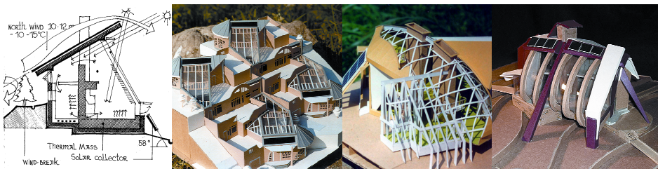
B. Passive and active solar heating study. Four year student’s project. Poster size 0.8 x 1.6 m., model. T.Belousova (1), E.Lezhenko (2), 2003.
